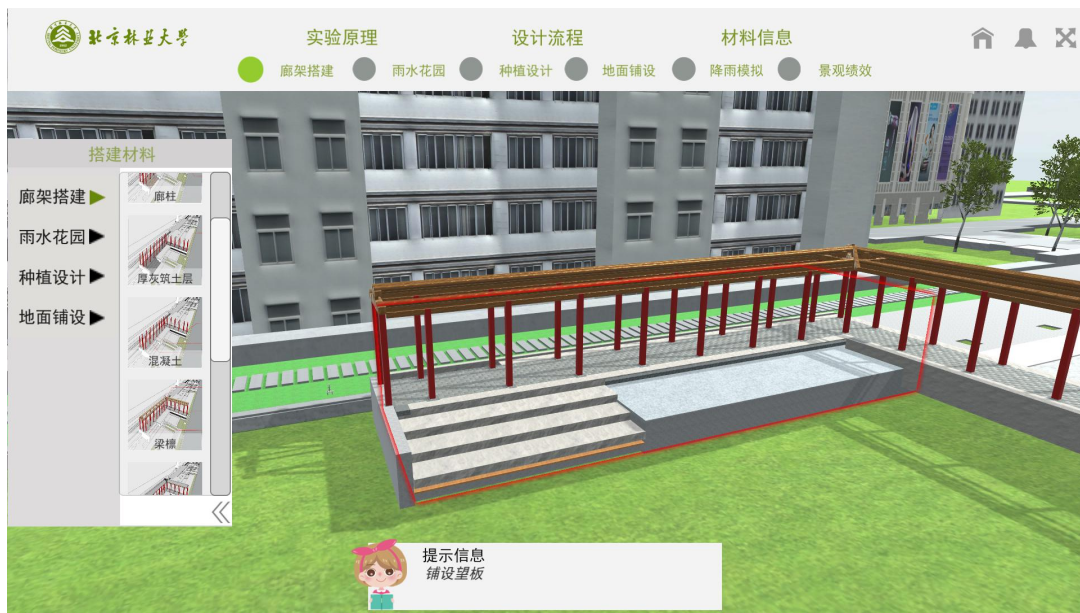
Figure 25 Construction of classical Gallery: beams and purlins
